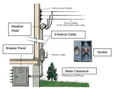
If a Field Service Representative observes a potential <u>Unsafe Condition</u> at your location: **loose, rusted, or worn meter socket, or worn entrance cable** that is in need of replacement or repair. This is an unsafe condition for you as a homeowner as well as the public. In addition, <u>Meter Clearance</u> **from bushes, vines, fences, or storage items** must be rectified before service is energized.
